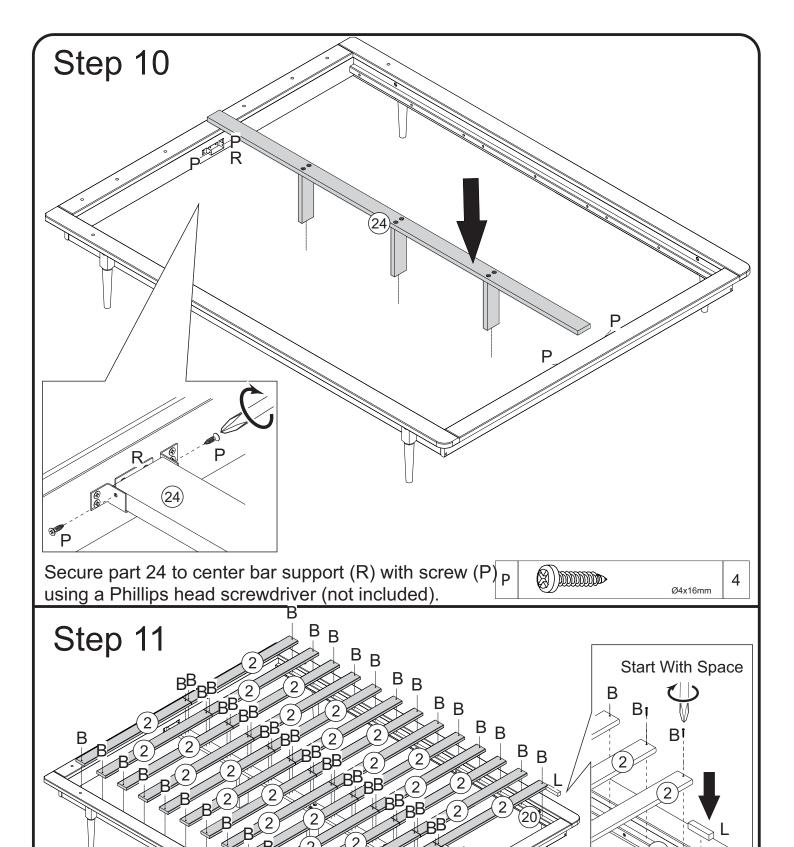
Place part 2 onto parts 20,24 and parts 21,24. Use part (L) to space part 2 from the end and secure with screw (B) using a Phillips head screwdriver. Move part (L) to space the next part 2, secure with screw (B), and repeat this process with the remaining parts 2.
