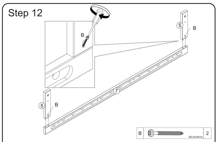
Connect parts 5 to part 7. Note the drawing for location of pocket hole. Secure parts 5 to part 7 with the screw (B) using a Phillips head screwdriver (not included).
