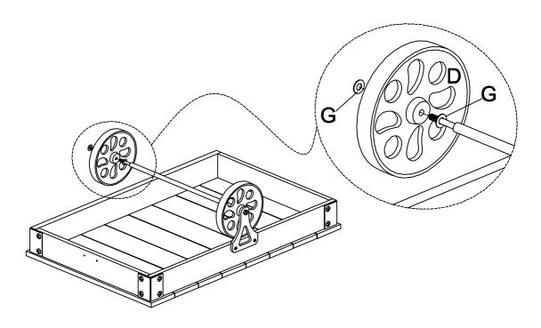
Attach the Big Caster (D) and Wheel Axle(E) as below showing to the Wheel Device(B) by using Washer (K) with Spanner (J), and then fixing the Wheel Device (B) to the Table Top (A) by using SpringWasher (H) and Bolt (F) with Allen Key (I).
