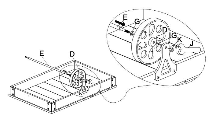
Attach the Big Caster (D) with Flat Washer (G) as below showing to the Wheel Axle (E).
