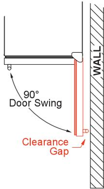
WHEN INSTALLING WITH THE HINGE SIDE NEXT TO A WALL - LEAVE ADEQUITE SPACE FOR CABINET HANDLES
