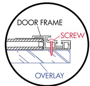
7 Using the (10) ST4-30 self-tapping screws supplied securely fasten
