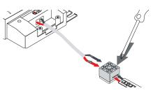
4. Use #1 Phillips to loosen the 4 terminal screws on 8MM-EZ Connector. Peel 1/2" of the adhesive protector from back of LED tape light, and scrape waterproof coating, insert into connector, evenly tighten screws. Insert wires from WAV Smart Receiver / Power Supply into terminals, Red wire to (+ or WW) side of tape, Black wire to (- or CW) side of tape; tighten screws.
