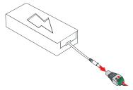
**4.** Insert Male Plug on power supply into Female Barrel Connector.
