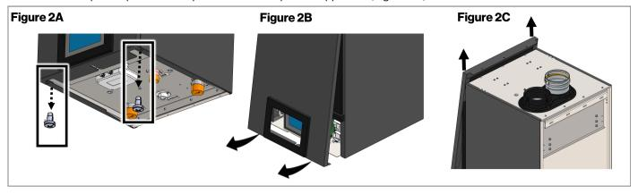
5. **RCB301AN/RCB399AN:** Use a Phillips head screw driver to remove three (3) screws holding left side panel (Figure 3A). Rotate the side panel out (Figure 3B), lift the panel up to clear the cutout located on back side of boiler, and remove the side panel (Figure 3C).
