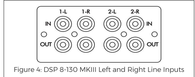
Figure 4: DSP 8-130 MKIII Left and Right Line Inputs
