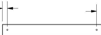
M21 | LISSE MURALE DU FORT - W4L12761 (x2) | 5/8 po x 3 3/8 po x 30 1/4 po (16x86x768)
