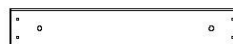
H77 | PLANCHE DE FIXATION - W4L14780 (x1) | 1 po x 3 3/8 po x 20 1/8 po (24x86x512)
