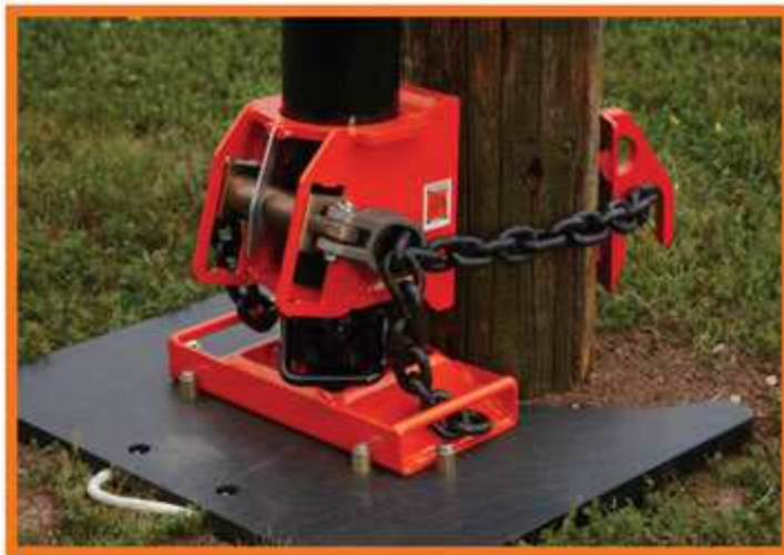
Swivel assembly pre-tensions the chain providing maximum lift per stroke.
