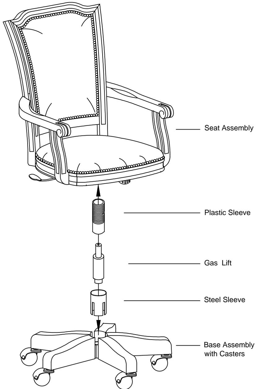
1. Position the Steel Sleeve into the Base Assembly.
