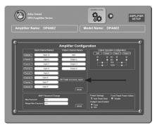
**DPA Amplifier Configuration Page** (Select Enable Accessory Inputs)
