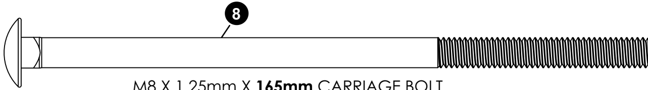
M8 X 1.25mm X 165mm CARRIAGE BOLT for poles up to 4" 1B-7258-00 QTY. 4
