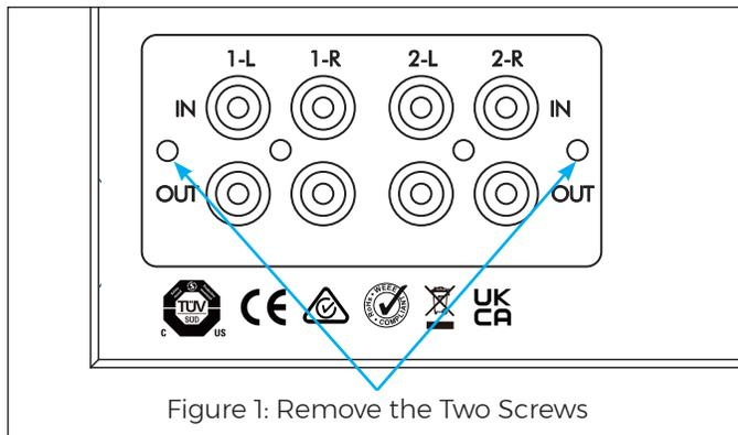
Figure 1: Remove the Two Screws
