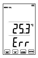
9. Touching the [ESC] key will navigate back 1 screen at a time. Calibration mode / then Menu mode, then HOME SCREEN. (If the reading is unstable or the sensor is not connected properly to the instrument, the "Err" sign will appear and blink 3 times on the screen and then return to the calibration menu.)
