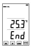
8. Once the calibration is completed, "End" will blink 3 times on the screen, indicating the desired calibration has been saved. The screen will then go back to the calibration menu. The device is now calibrated.
