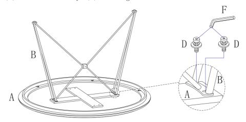
Attach the Leg (C) to the Leg (B) and the Table Top (A), using Flat Head Bolt (E), Bolt With Lock Washer And Flat Washer (D) and Allen Key (F) to tighten.
