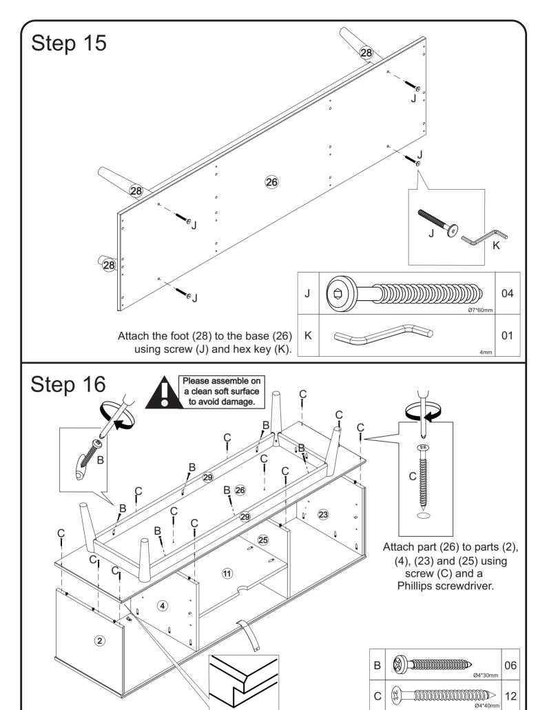
Attach the part (29) to the base (26) using screw (B) and Phillips head screwdriver.
