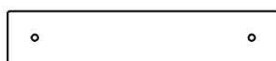
M18 | LISSE MURALE - W4L16053 (x1) | 5/8 po x 3 3/8 po x 16 7/8 po (16 x 86 x 430)
