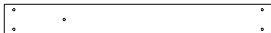
G10 | LISSE DE PLANCHER - W4L16010 (x1) 1 po x 5 1/4 po x 45 1/2 po (24 x 134 x 1156)
