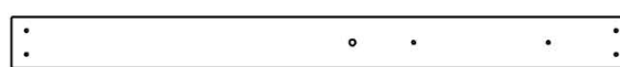
M17 | PANNEAU MURAL - W4L16090 (x2) | 5/8 po x 3 3/8 po x 41 po (16 x 86 x 1040)
