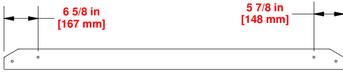
AD02 WALL RAIL - W4L21401 (x2) 1"x3 7/8"x65 3/4" (24x100x1670)
