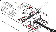
3. Insert one end of stripped wires into WAV Smart Receiver LED Terminals, Red wire to (WW+) and Black wire to (CW-) terminals. Tighten screws.
