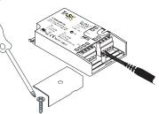
2. Use #2 Phillips to loosen screw and remove cover from WAV Smart Receiver. Use the flat head from the multi-bit screwdriver to loosen one terminal marked (CW-) and one marked (WW+).
