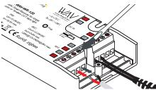
Insert one end of stripped wires into WAV Smart Receiver LED Terminals, Red wire to (WW+) and Black wire to (CW-) terminals. Tighten screws.
