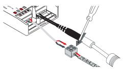
4. Use #1 Phillips to loosen the 4 terminal screws on 8MM-EZ Connector. Peel 1/2" of the adhesive protector from back of LED tape light, and scrape waterproof coating, insert into connector, evenly tighten screws. Insert wires from WAV Smart Receiver into terminals, Red wire to (+ or WW) side of tape, Black wire to (- or CW) side of tape; tighten screws.
