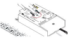
2. If setting WAV Smart Receiver up for the first time, clear the memory by pressing and holding the "Prog" button until the lights blink twice.
