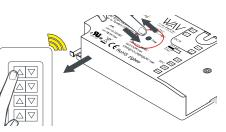
3. Very quickly, click and release the "Prog" button and, within 5 seconds, quickly click and release the "On Light Bulb" button on the Controller. When lights blink once, Controller and Receiver are paired.
