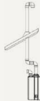
Vertical termination room air configuration
