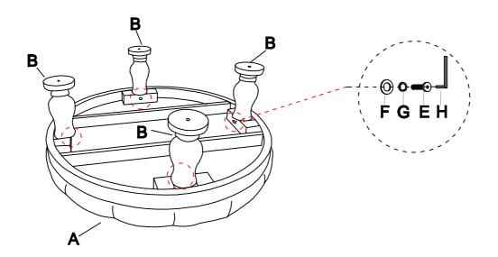
Attach Bottom(C) to Leg(B) by using Bolt(D), Flat Washer(F), Spring Washer(G) and Allen Wrench(H) as shown.
