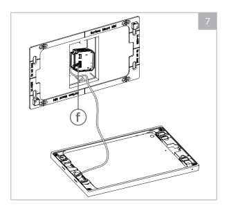
Connect the appropriate power source identified in the Power and Wiring Guide (found in (f) PoE+ Adapter box). Place the PoE splitter into the single gang box located in the wall.
