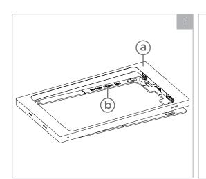
When removing the Surface Mount (a) bezel from its box, the bezel will be attached to the (b) mounting bracket. To decouple the (a) bezel from the (b) mounting bracket, place the (a) bezel face up on a flat and smooth surface. With one hand, hold the (b) mounting bracket in place. With your opposite hand, lift the right edge of the (a) bezel and then the left to decouple the magnets. This will help avoid bending of the metal, and prevent any damages to the (a) bezel or (b) mounting bracket.
