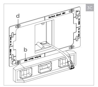
Level the (b) mounting bracket over wiring location and fasten (b) bracket with the remaining (d) screws. Lining up the (d) mounting screws with the engraved center lines provided on the (b) bracket will allow optimal adjustability. The (b) mounting bracket is now in place.
