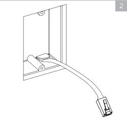
Locate the ideal mounting area. For retrofit installation, locate an existing low-voltage electrical box. For new construction, choose a location for an electrical box. We recommend installing the (a) bezel in landscape orientation, but it can also be installed in portrait orientation.
