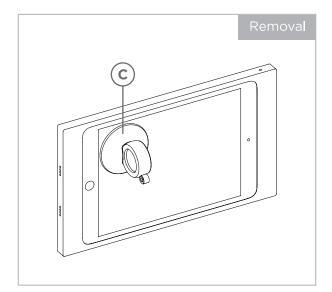
The (c) suction cup (provided) is used to remove the iPad and (a) bezel from the (b) mounting bracket. Once the (a) bezel is unlocked from the (b) mounting bracket, depress the (c) suction cup on the corner of the iPad screen and carefully pull the iPad from the wall, while the other hand is supporting the opposite side of the (a) bezel.
