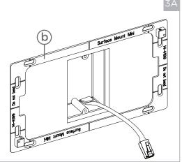
Install the (b) mounting bracket on the wall with the (b) bracket surrounding the electrical box. Use the center lines as a guide to install the (d) mounting screws. The IPORT specialized (d) mounting screws act as anchors and screws when mounting on a drywall or wood surface.
