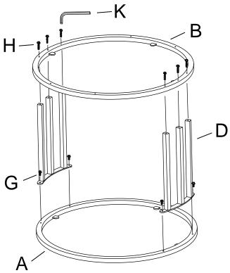
Attach two side panels (D) to middle frame (B) by bolt (G) and allen wrench (K). Attach bottom frame (C) to side panel (D) by bolt (H) and allen wrench (K) as shown.
