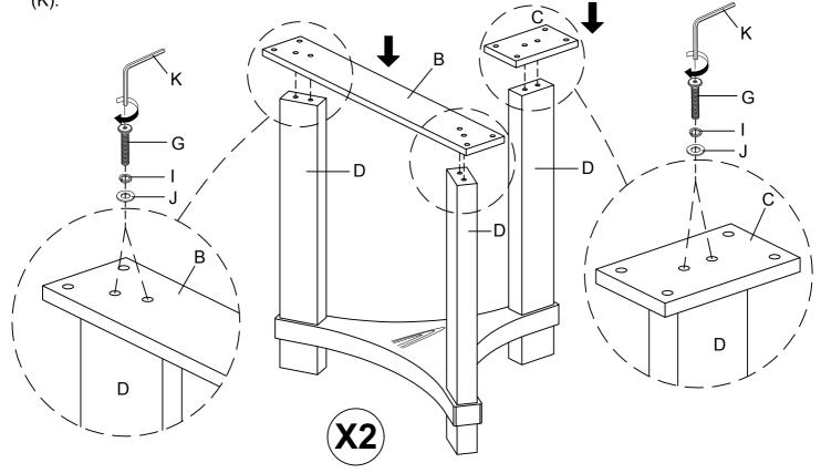
Attach the Long Mounting Plate (B) and the Short Mounting Plate (C) to the Table Top (A) using Allen Bolt (G), Lock Washer (I) and Flat Washer (J) with the Allen Key (K).
