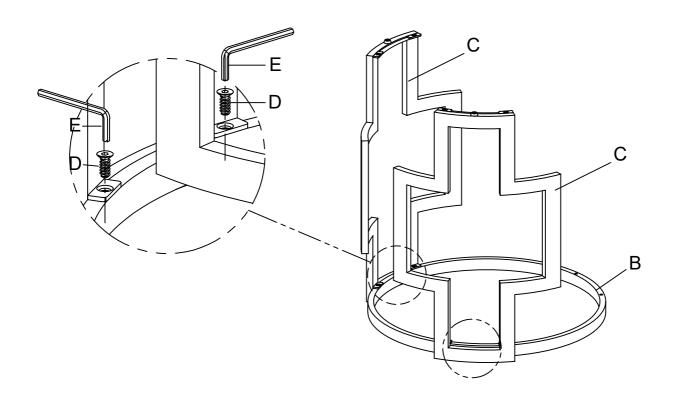
Attach pre-assembled Side Frame (C) to the rest 1pc of Top & Bottom Frame (B) using Bolt (D) by Allen Key (E) as below shown.
