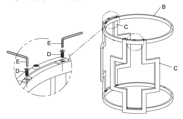
Attached the rest 1pc of Side Frame (C) to Top & Bottom Frame (B) using Bolt (D) by Allen Key (E) as below shown.
