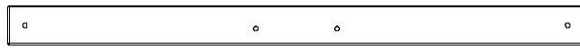
H14 | SUPPORT DE POUTRE DE BALANÇOIRE - W4L12719 (x1) | 1 po x 3 3/8 po x 50 1/4 po (24x86x1277)
