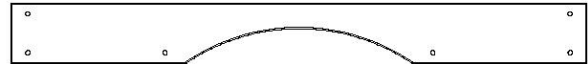
K5 | LISSE MURALE DU PAVILLON - W4L14785 (x1) | 5/8 po x 5 1/4 po x 50 1/4 po (16x134x1277)
