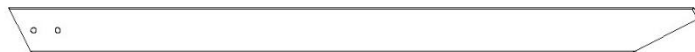
H81 | CALE DE BARRE DE SUSPENSION - W4L15710 (x2) | 1 po x 3 3/8 po x 51 5/8 po (24x86x1311)
