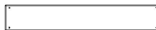
L1 | PLANCHE DE PLANCHER DU NID-DE-PIE - W4L14787 (x8) | 5/8 po x 4 3/8 po x 27 po (16x112x686)
