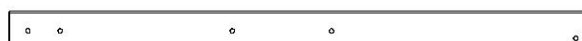
H10 PIED DU PORCHE - W4L14757 (x1) | 1 po x 3 3/8 po x 50 1/2 po (24x86x1282)
