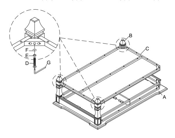
Attach the last Legs (B) to the Top Panel (A) & Bottom Panel (C) using Bolt (D), Lock Washer (E) and Flat Washer (F), on holes of Top Penal (A) and Bottom Panel (C) by Allen Key (G). Turn the
