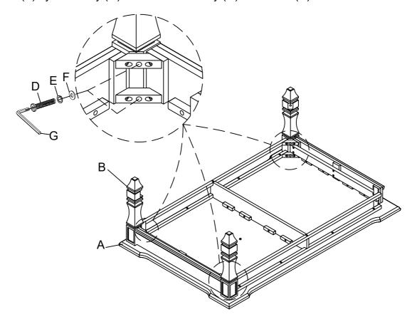
Attach Bottom Panel (C) to the three Legs (B) using Bolt (D), Lock Washer (E) and Flat Washer (F), on holes of Bottom Panel (C) by Allen Key (G). Turn the Allen Key (G) in the Bolt (D).
