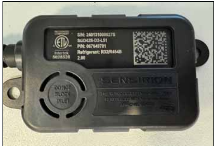
FIGURE 21. Example of Clear, Unobstructed Sensor Inlet
