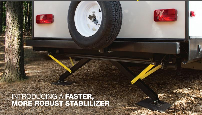
New for 2019, the PSx2 Stabilizer adds several improvements to the PSx1 Stabilizer which was first introduced in 2005. Easily retract and extend the jacks with the flip of a switch. In just a few minutes, the coach will be stable, so you can spend less time setting up camp and more time enjoying your vacation. Power Stabilizer Jacks are an affordable way to upgrade to power stabilization and easily bolt on to the existing frame.
