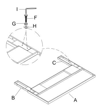
Attach Left Side Panel (D) & Right Side Panel (E) to Headboard (A) using Flat Washer (H), Lock Washer (G), Bolt (F) by Allen Key (I).
