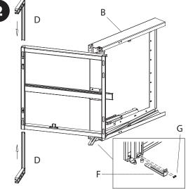
Insert door brackets into side frame and secure with (4) machine screws finger tight at this time. Install L shaped part of swivel arm onto bottom of axle using (2) provided pan head machine screws (see drawing)
