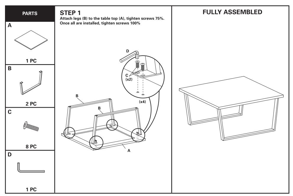
NOTE: DO NOT TIGHTEN SCREWS UNTIL COMPLETELY ASSEMBLED
