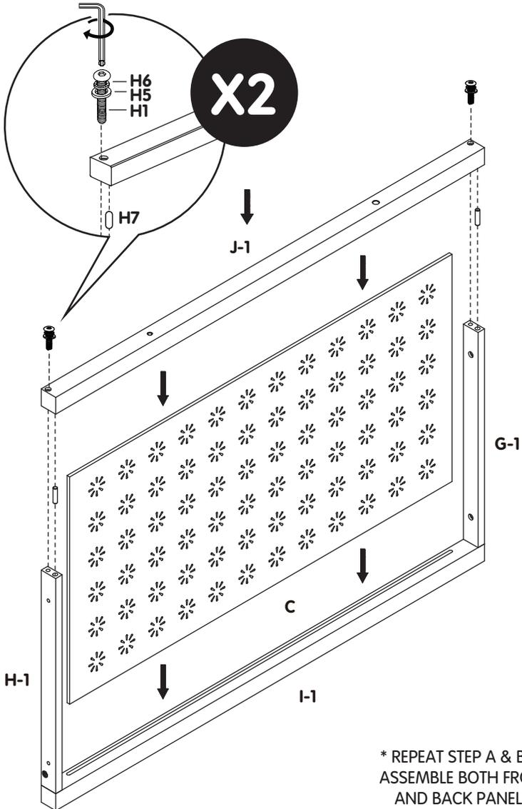
\* REPEAT STEP A & B TO ASSEMBLE BOTH FRONT AND BACK PANELS.
