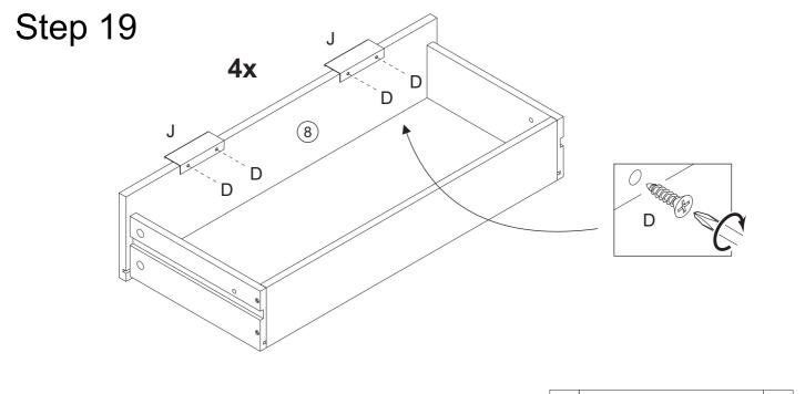
Secure handle (J) with screw (D) and phillips head screwdriver,
