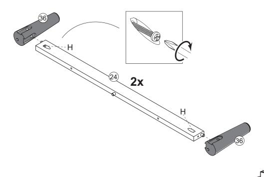
Secure part 24 to parts 36, with screw (H) and phillips head screwdriver.
