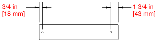
M2 | WALL RAIL - W4L06393 (x2) | 5/8"x3 3/8"x17 1/2" (16x86x445)
