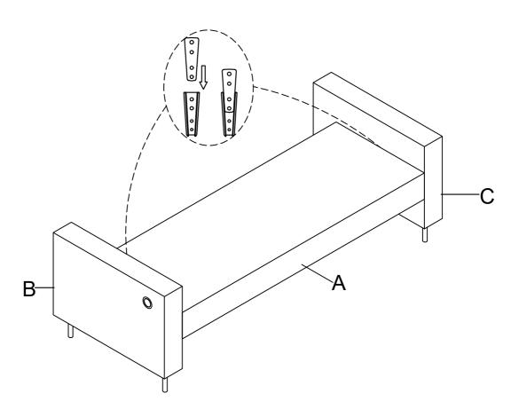
4 Hook on the Back Rest (D) to the Seat Frame (A), Left Arm (B) and Right Arm (C) properly.
