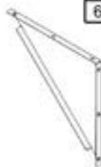
A11 PANNEAU TRIANGULAIRE- A4M03086 (x2) 13/16"x13 3/4"x13 3/4" (20x350x350)
