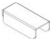
A5 SUPPORT D'ÉTAGÈRE - A4M03141 (x8) 5/8"x7/8"x2 1/16" (16x22x53)
