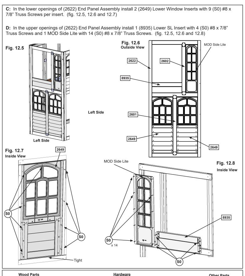
2 x 2649 Lower Window Insert 1.27 x 18.8 x 41.91" 1 x 8935 Lower SL Insert 1.36 x 8-1/8 x 26-1/4" (from TNR III box) 36 x (so) #8 x 7/8" Truss Screw
