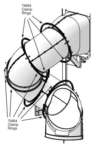
Note: For ease of assembly the bottom set of clamp rings can be turned 90 degrees to install bolts.
