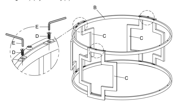
Attached the rest 1pc of Side Frame (C) to Top & Bottom Frame (B) using Bolt (D) by Allen Key (E) as below shown.
