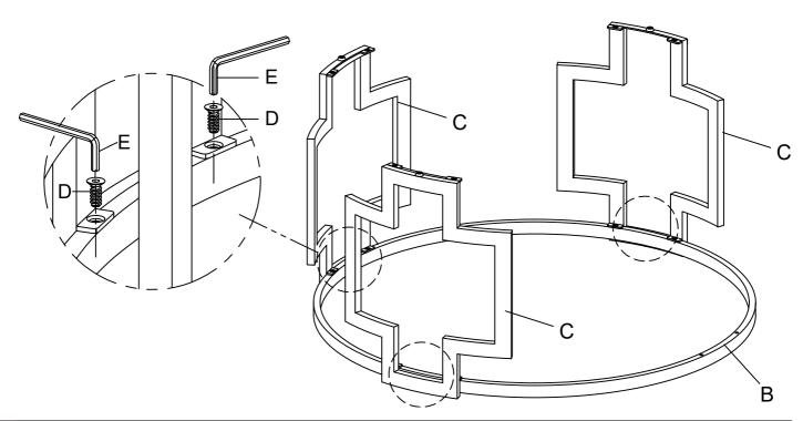
Attach pre-assembled Side Frame (C) to the rest 1pc of Top & Bottom Frame (B) using Bolt (D) by Allen Key (E) as below shown.
