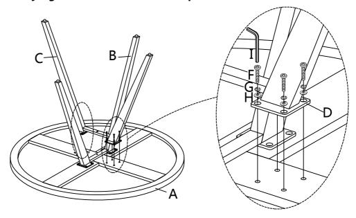
Use Long Bolt (F), Spring Washer (G), Flat Washer (H) with Allen Key (I) to fix Upper Leg Frame (B) and Lower Leg Frame (C).
