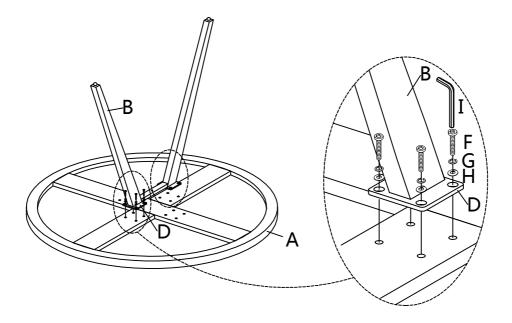
Attach Lower Leg Frame (C) to Upper Leg Frame (B) and bottom of Top Panel (A) using Long Bolt (F), Spring Washer (G), Flat Washer (H) with Allen Key (I).
