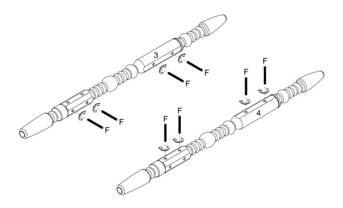
Now let's finish the headboard! Insert the bolts in the Headboard Posts (3 & 4) into the Headboard (1) and Headboard Rail (2). To secure, put the Half Moon Washer (G) over bolt in the circle openings on the Headboard (1) and then tighten the Nut (H) on top with the Wrench (J).
