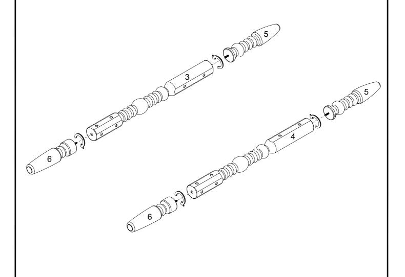
Next, twist in the Bolts (F) to the Left and Right Headboard Posts (3 & 4). For now, leave the four holes in the image without bolts empty.
