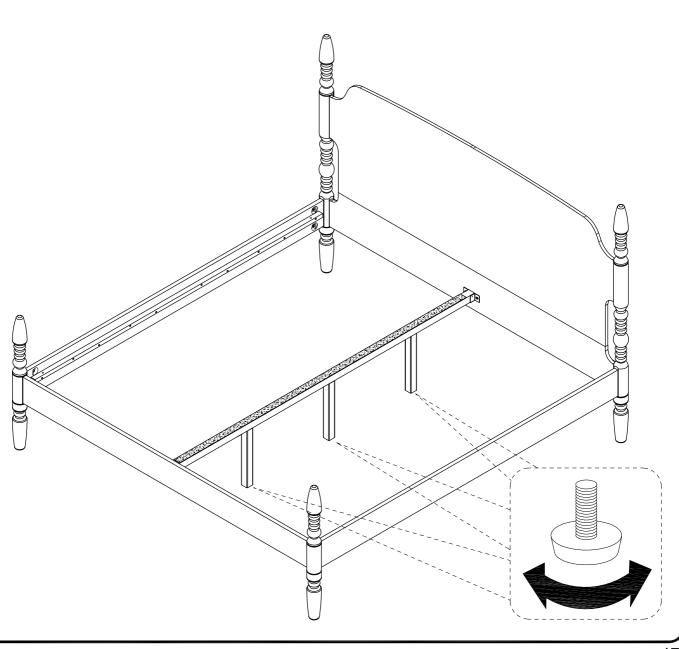
Place the dowels (B) into the holes on each end of the Side Rails (7), this will help when aligning the slats.
