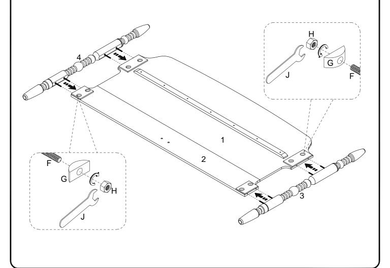
Turn the assembled headboard over and twist in Bolts (F) to the front side of the Left and Right Headboard Posts (3 & 4). Also attach the U Bracket (K) to the Headboard Rail (2) with a Washer(D) and Bolt (C).
