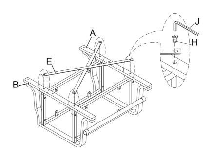
Assemble Connect Bar (F) to Side Frame - LSF (A) & Side Frame - RSF (B), using Bolt (H) by Allen Key (J), then put Plastic Cap (M) to the bottom of Side Frame - LSF (A) & Side Frame - RSF (B) as below shown.
