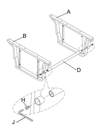
First, assemble Shelf Frame (C) to Side Frame - LSF (A) & Side Frame - RSF (B), using Bolt (H) by Allen Key (J) as below shown.
