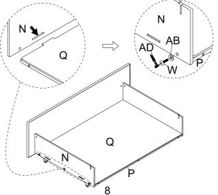
Attach the Drawer Back Board (O) to the Drawer Bottom Frame (P), insert the Bolt (W) and Washer (AB), turn the Ratchet Tool (AD) to tighten them. Attach the Drawer Board Connector (R) to the assembled drawer, insert them into correct places.
