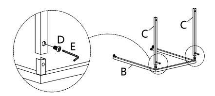
Insert Leg (B) to Rail (C) using Bolt (D) with Allen Key (E).
