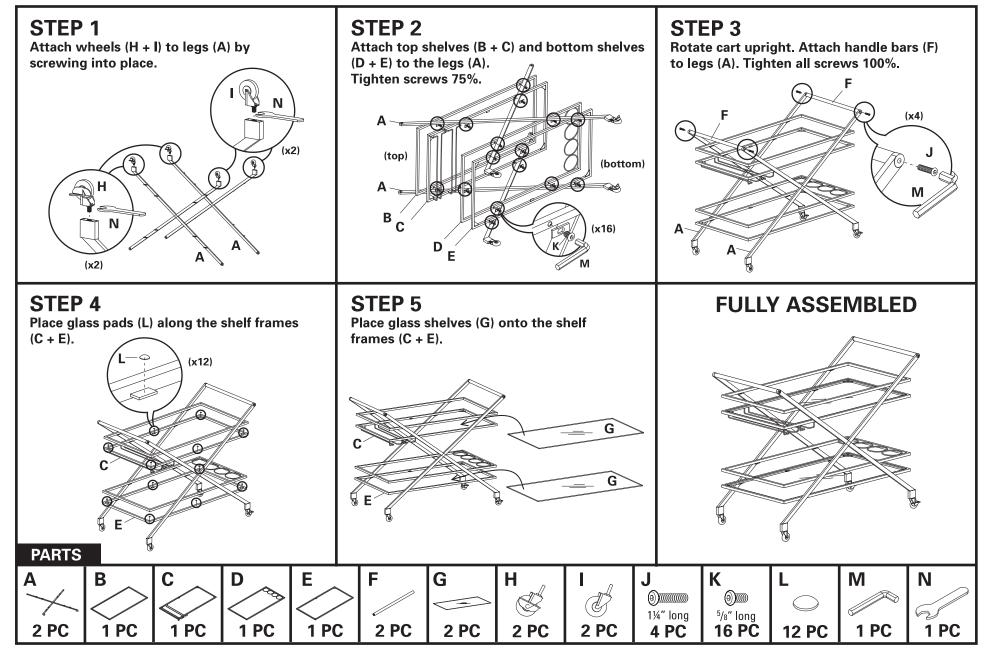
NOTE: DO NOT TIGHTEN SCREWS 100% UNTIL FULLY ASSEMBLED.
