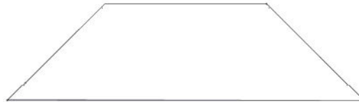
R02 ROOF COVER - W4L22340 (x1) 3/16"x23 7/16"x85 13/16" (5x595x2179)
