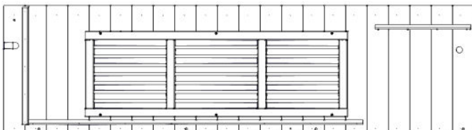
P10 RIGHT WALL PANEL - W2A04907 (x1) 2 3/8"x19 5/8"x72 13/16" (61x499x1850)
