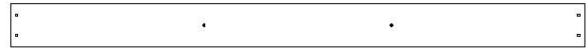
M01 PLANCHE DE PLANCHER - W4L16120 (x1) 5/8 po x 3 3/8 po x 44 7/8 po (16x86x1140)
