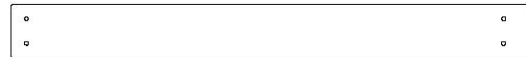
G02 RAIL AU SOL - W4L16129 (x1) 1 po x 5 1/4 po x 51 1/8 po (24x134x1300)
