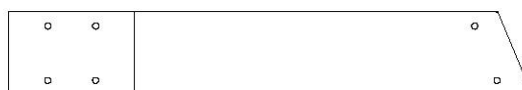
G07 RAIL AU SOL - W4L16165 (x1) 1 po x 5 1/4 po x 32 3/4 po (24x134x832)
