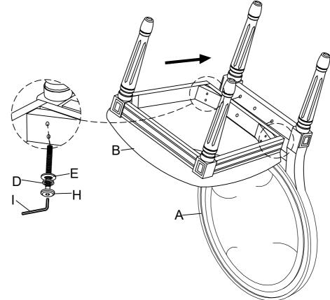
Finally, assemble the last Bolt (F) to Seat (B) and Chair Back (A) with Lock Washer
