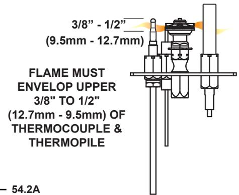
FLAME MUST ENVELOPE UPPER 3/8" TO 1/2" (12.7mm - 9.5mm) OF THERMOCOUPLE & THERMOPILE
