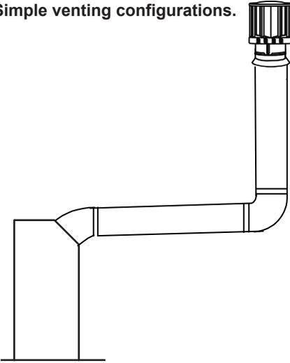
See graph to determine the required vertical rise  $V_T$  for the required horizontal run  $H_T$ .
