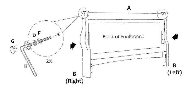
Insert JCBC Bolt (C), Spring Washer (F) and Flat Washer (E) to the holes at the back of Foootboard and tighten using Allen Key (H).
