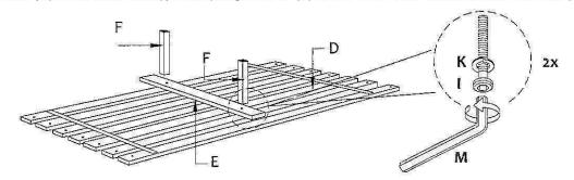
Turn the Slats (D) and place it to the Side Rail (C). Tighten the Slats (D) with CSK Screw (L) using Phillip Head Screwdriver (Not provided).
