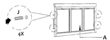
Attached Headboard Leg (B) to the Headboard Panel (A). Insert JCBC Bolt (E) and Spring Washer (G) to the holes and fighten using Allen Key (I). Cover the holes with Wooden Button (H). Attached Bottom Rail Support (C) to Headboard Leg (B). Insert JCBC Bolt (D), Spring Washer (G) and Flat Washer (F) to the holes and fighten using Allen Key (I).
